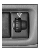
The thumbwheel for this feature is located to the left of the steering wheel on the instrument panel.
